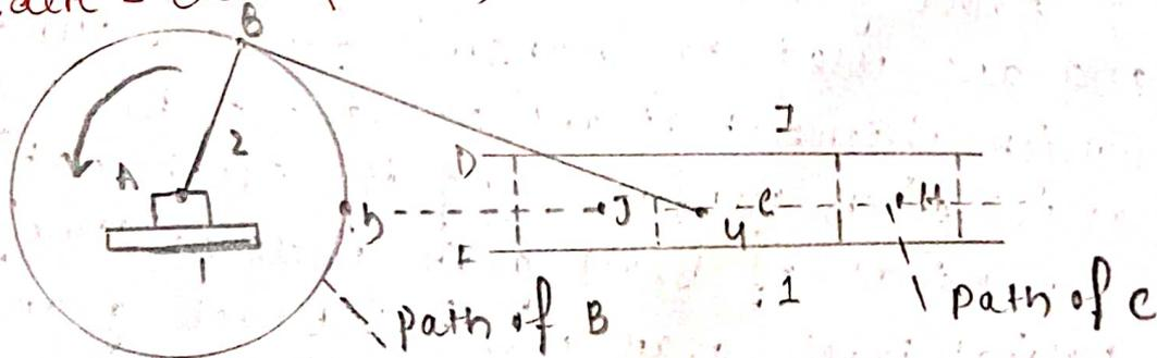
Slider - crank mechanism, arrangement of mechanical parts designed to convert straight line motion to rotary motion, as in a reciprocating piston engine, or to convert rotary motion, as in a reciprocating piston pump.
