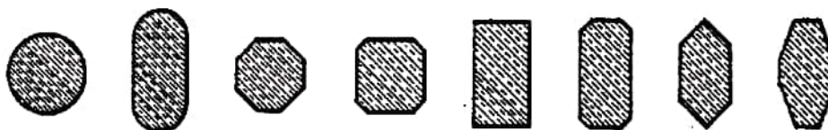
FIGURE: 1 : Typical cross-section shapes of piers for overcrossings or viaducts on land.
